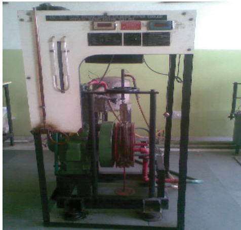
Plate 1. Single Cylinder Diesel Engine
