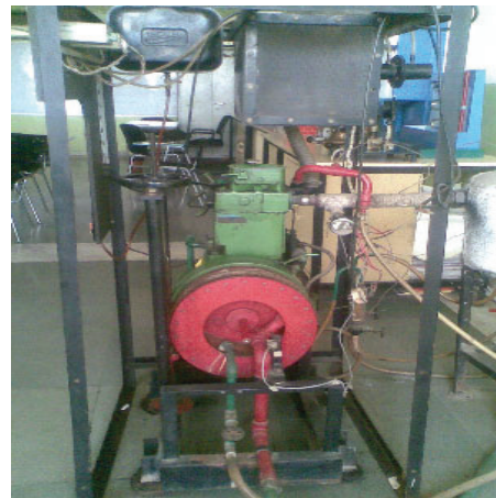
Plate 2. Rope Drake Dynamometer
